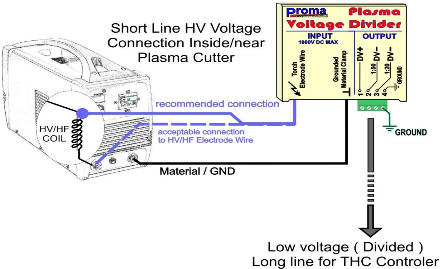
In order to minimize interference and the possibility of overvoltage it is recommended to connect the divider before the HF/HV generator by connecting the blue (electrodes) in front of the coil of the HV/HV generator. There are much smaller HF/HV voltage interferences here.
