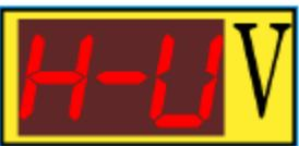
**"H - U" (High Voltage)** - value of the off load voltage detection in the plasma cutter - used to detect the main (cutting) arc: 50-300V by default: 200V
