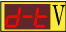
**"d - t" (delay time)** - delay time of output closed despite no supply voltage, when the system detects the main (cutting) arc 0.1 - 9.9s factory setting: 0.5s
