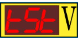
**"tSt" (Test)** - Simulation of the controller's work - the system simulates the appearance of "floating" voltage within the selected value - causes the activation of inputs for easy system testing without switching the cutter on.
