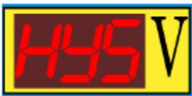
**"HYS" (Hysteresis)** - The hysteresis voltage - a range in which the voltage is measured, in which there are signals controlling UP/DOWN 2-30V ( $\pm 1V$  -  $\pm 15V$ ) - factory setting: 8V ( $\pm 4V$ )
