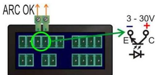
ARC OK output (confirmation of the main arc ignition) is the optically insulated OC output (open collector). The output is active (closed) when the main arc has been detected.
