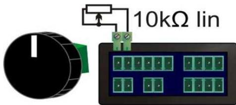
The input supports 10kΩ potentiometer and is used for fast and convenient adjustment of the preset voltage by +/- 15V.
