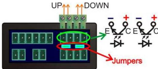
The UP / DOWN outputs are OC optically insulated outputs (open collector). The maximum voltage that can be connected to the UP /
