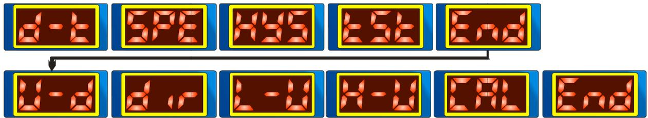
**6.1 Starting the controller** should begin by connecting **ONLY** the power supply (**point 5.1**) and initial configuration of key service parameters. First, select the operating mode of the controller - **THC SD (default)**, or THC 150. For this purpose, when supplying the power-hold both UP /
