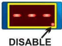
DISABLE INPUT CONTROL: When DISABLE signal is active last dot on display is lighting.
